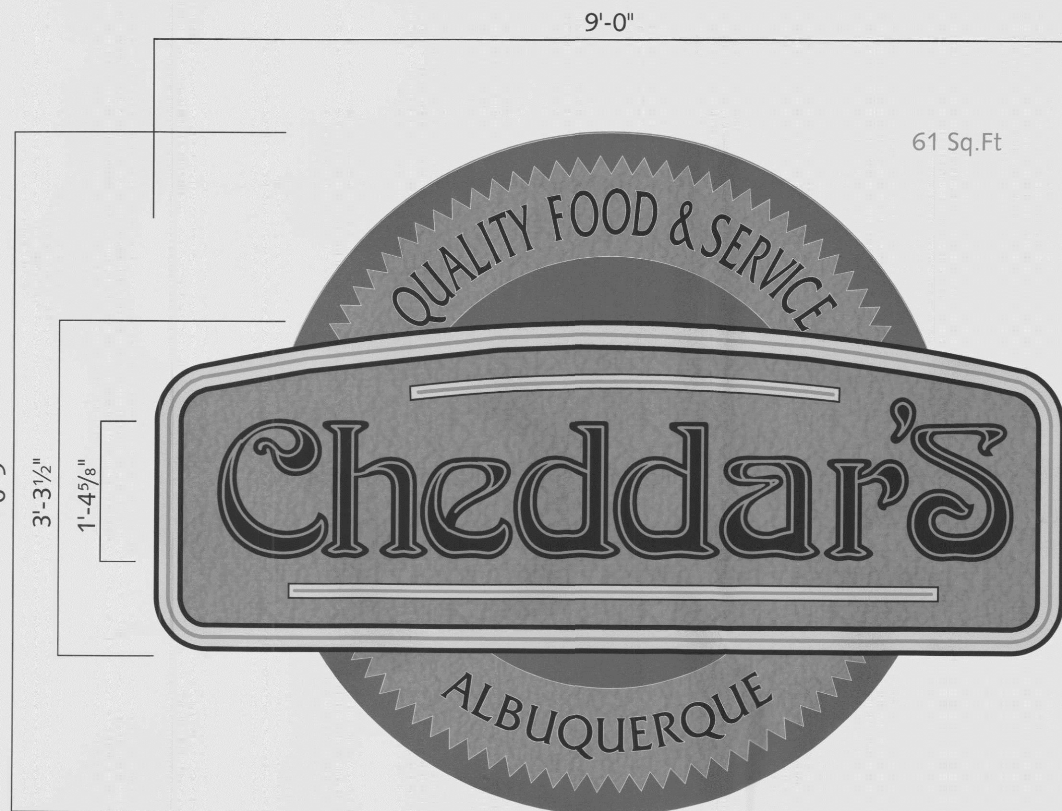
B S/F WALL SIGN ELEV. - MAIN I.D. SCALE: 1/2" = 1'-0" ( 1 ) REQUIRED - MANUFACTURE AND INSTALL
