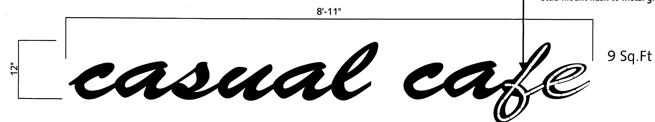
FCO LETTER LAYOUT (FLAT VIEW) SCALE: 1/2"=1'-0" MFR. AND INSTALL ( 1 ) SET FCO LETTERS WITH S/T NEON ON RADIUS METAL GRID
